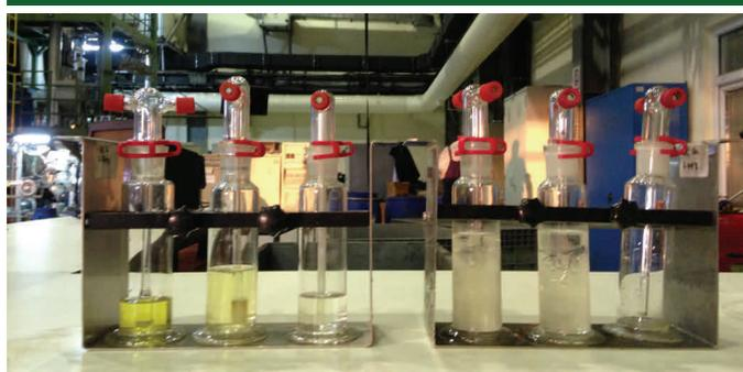
Figure 3: Tar samples collected from an air gasification study using a bubbling fluidised bed gasifier.
